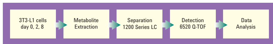
Figure 2. Workflow for the analysis of the lipidome of 3T3-L1 cells at days 0, 2, 8. Lipids were isolated using the Folch [1] extraction method, followed by LC-MS analysis and data analysis using GeneSpring MS.
